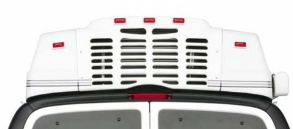
A 'Dometic' heat pump (air conditioner & heater) built into a recess in the roof cools the interior while maintaining Chevy based Roadtreks' aerodynamic shape and sleek roofline. In many restricted communities, vehicles with roof mounted air conditioners are not permitted. Our recessed heat pump allows our Chevy based motorhomes to be perceived as just vans and in most cases are permitted to park where many other motorhomes are not.
