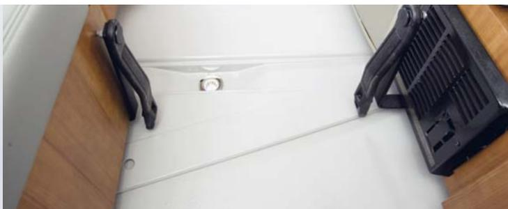
A removable cover in Chevy based Roadtreks reveals a trough with a drain that spans the lowered floor and prevents water from leaving the shower area.
