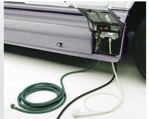
There is a separate compartment for the city water connection with quick disconnect and detachable power cord for trips away from the campsite. An exterior shower is located here as well.
