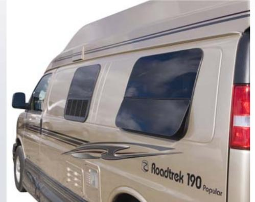
Frameless awning windows are better looking, reduce wind noise, improve aerodynamics, and provide superior air circulation even during foul weather. Their larger size provides a better view from inside. The Integrated Venting System (most Chevy models) provides inconspicuous ventilation of the refrigerator.
