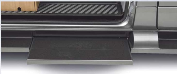
RS and SS models feature a power step at the side entry that extends/retracts with the opening and closing of the sliding entry door. An override switch allows the step to be left extended while parked. Sensors ensure the step retracts when driving.
