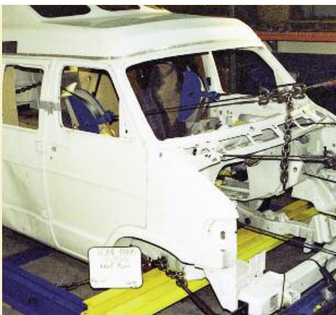
These 2 photos depict simultaneous seat belt pull testing and seating system testing. Seat belt testing confirms proper seat belt location and minimizes the possibility of anchorage failures. Seating system testing verifies the integrity of the seats, their attachments, mounting hardware and installation.
