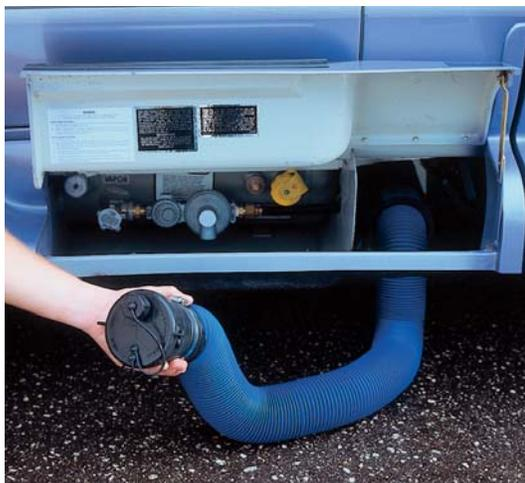
Easily accessible by flipping up the driver's door step, our patented "Dura Drain" sewage hose system provides a permanently attached sewage hose that eliminates messy handling and storage. Also located here are the waste water tank releases, LP gas fill and gauge plus the fresh water tank drain.
