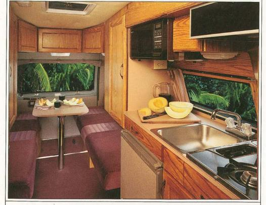
16. (Top) 190-Versatile, 190-Independent or 210-Independent galleys are fully equipped with a 'Dometic' 3.0 cu. ft. 3-way refrigerator, 'Panasonic' variable intensity microwave oven, LP gas stove, exhaust fan, sink, monitor panel and LP gas detector. 210-Independent also features another full length wardrobe or pantry (via removable shelves) and much more counter and cabinet space. In all models, a spacious eating
