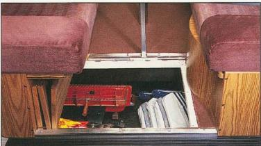
14. Additional storage space is supplied within our unique storage trunk located beneath the floor at the rear of the unit.
