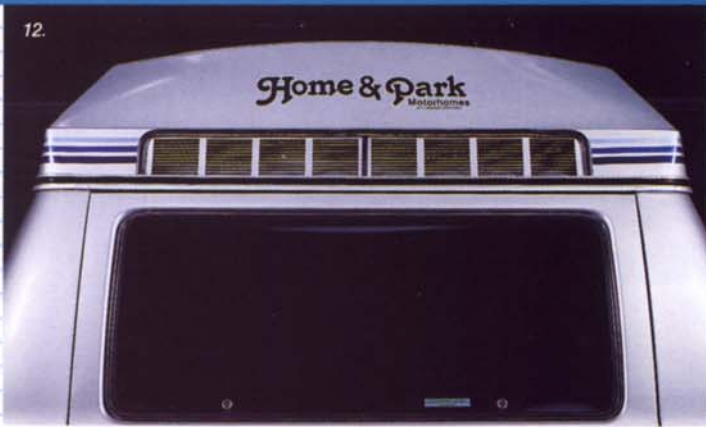
A 110V air conditioner built into the upper rear cupboard (see 9) maintains Roadtrek's low roofline. Only an inconspicuous grill is externally visible.
