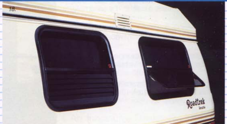
Integrated venting system (left) allows ventilation of the appliances while maintaining an aesthetic appearance. Awning windows provide superior air circulation during foul weather without soaking the interior.
