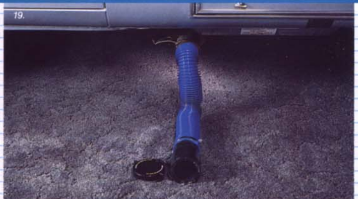
Patented 'Dura-Drain' sewage hose system provides a permanently attached built-in sewage hose that eliminates sewage hose handling and storage inconvenience.
