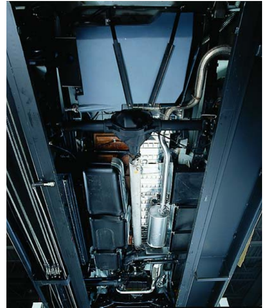
Water tanks fit below the floor which maximizes interior storage space and improves weight distribution for better handling.
