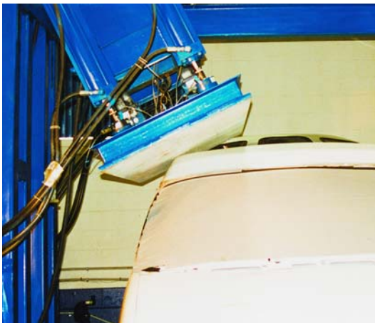
Roof crush resistance testing is intended to reduce death and injuries from roof crushing during rollover accidents.
